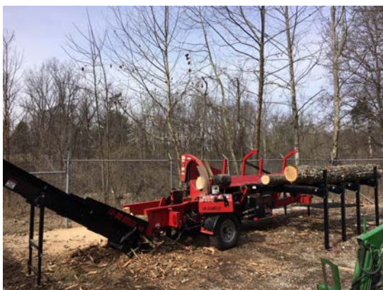
Firewood processor helps fuel facilities and produce campfire wood at Starve hollow SRA
