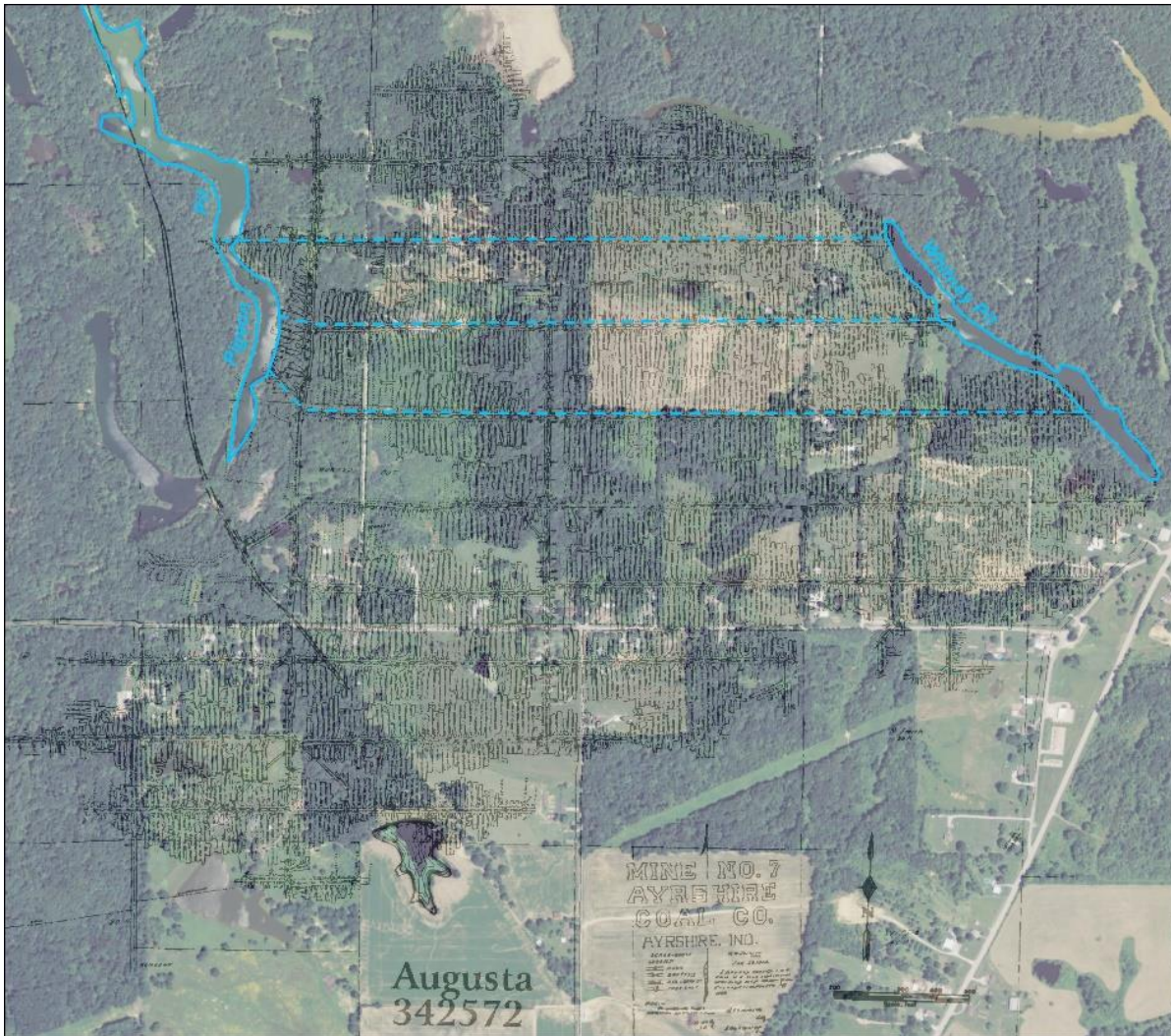
Map of Whitney and Pigeon Pits superimposed with a map of the Ayrshire #7 underground mine. The mine void created a direct connection between the two pits, which created a substantial challenge during the reclamation of Pigeon Pit in 2016 as part of the Sugar Ridge #2 project. Buttermilk Pit (unmarked, upper center right of map) was also hydrologically connected to the mine, although the response to that pit to pool level changes in the mine was not as abrupt.
