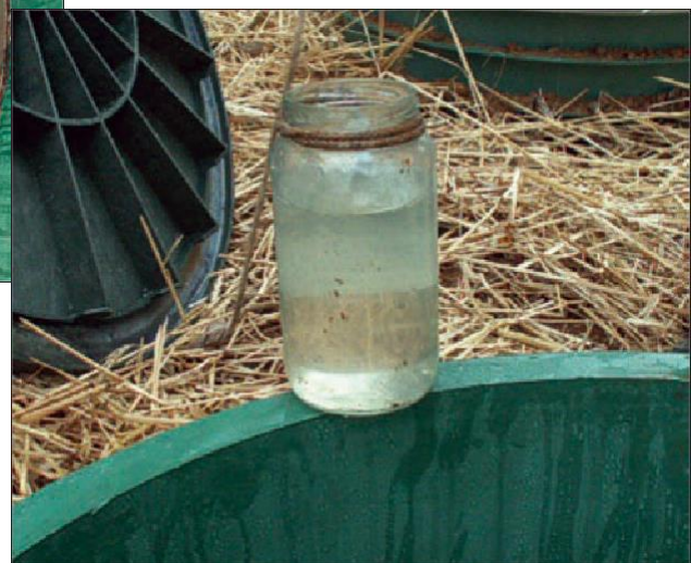
Sample of treated effluent pulled from the discharge side of the Model 1200 pods.
