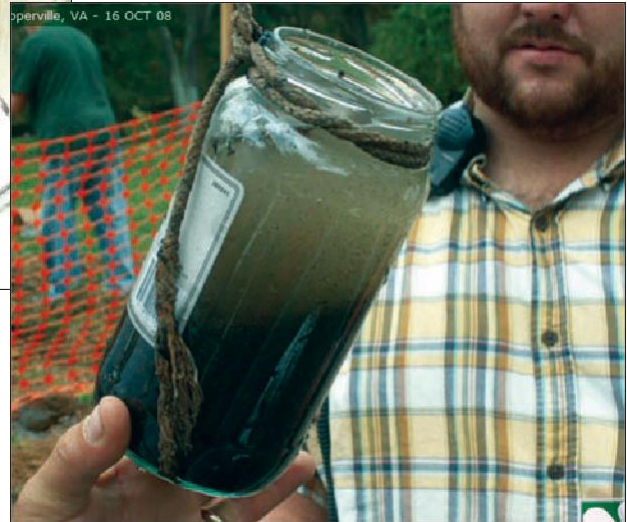
Sample pulled from the discharge side of the High Strength Aerobic Treatment Unit.
