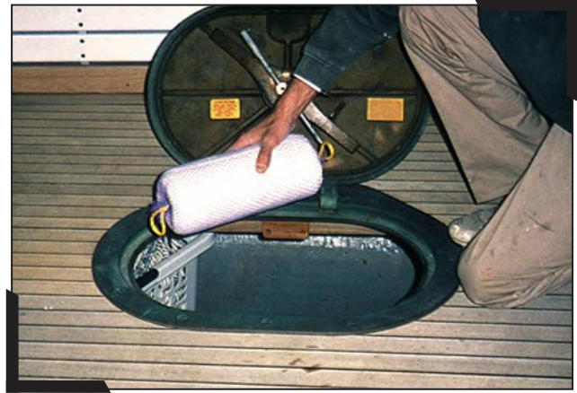
Use bilge socks to absorb oil (Source: Jay Tanski, New York Sea Grant).
