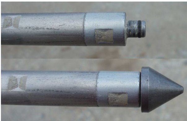
Figure 13-2 No Tip Installed (Top) Disposable Tip (Bottom)
