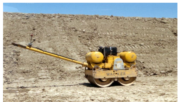
Figure 4-5 Hand Vibratory Roller
