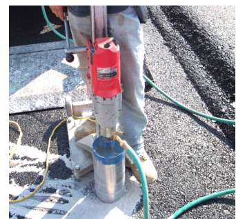
Figure 7-9 Taking an HMA Core Sample
