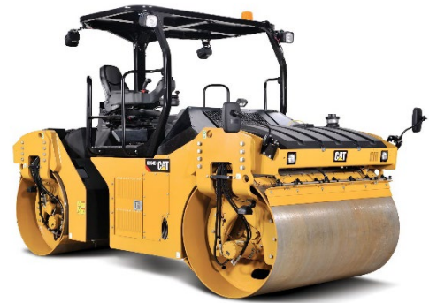
Figure 3-8 Two-Axle Tandem Roller
