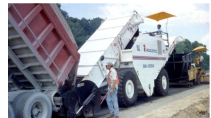
Figure 3-15 Material Transfer Vehicle
