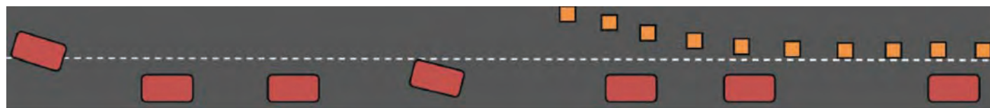
Figure 3.1. Illustration of early-merge concept (Credit: FHWA).
