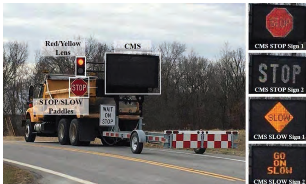
Figure 2.14. Missouri AFAD with changeable message sign (Credit: University of Missouri).
