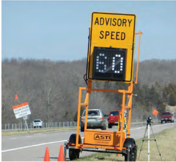
Figure 2.6. Advisory PVSLS trailer at a Missouri work zone (Credit: University of Missouri).
