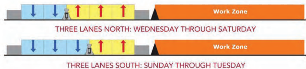
Figure 3.8. I-75 reversible lane setup (Credit: Lindsay Corporation).
