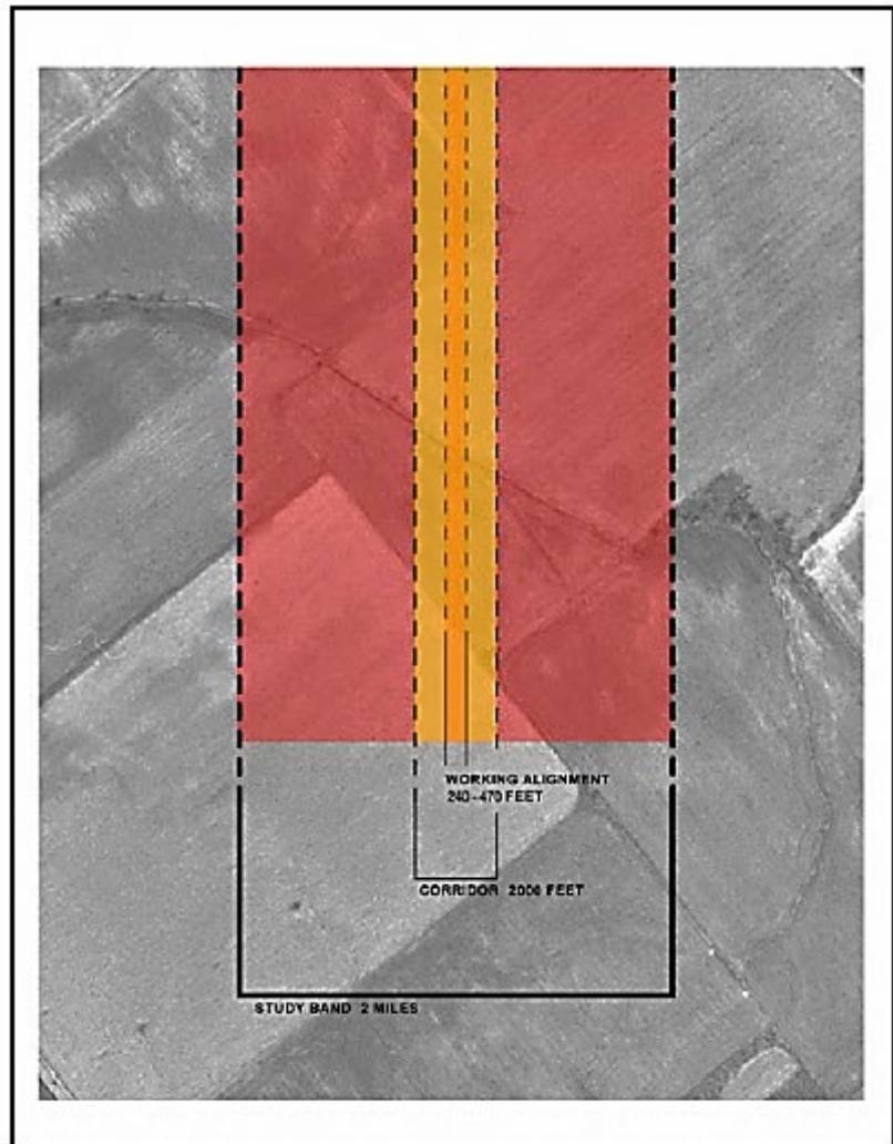
Figure 5.1-1: Study Band, Corridor, Working Alignment (Tier 1)
